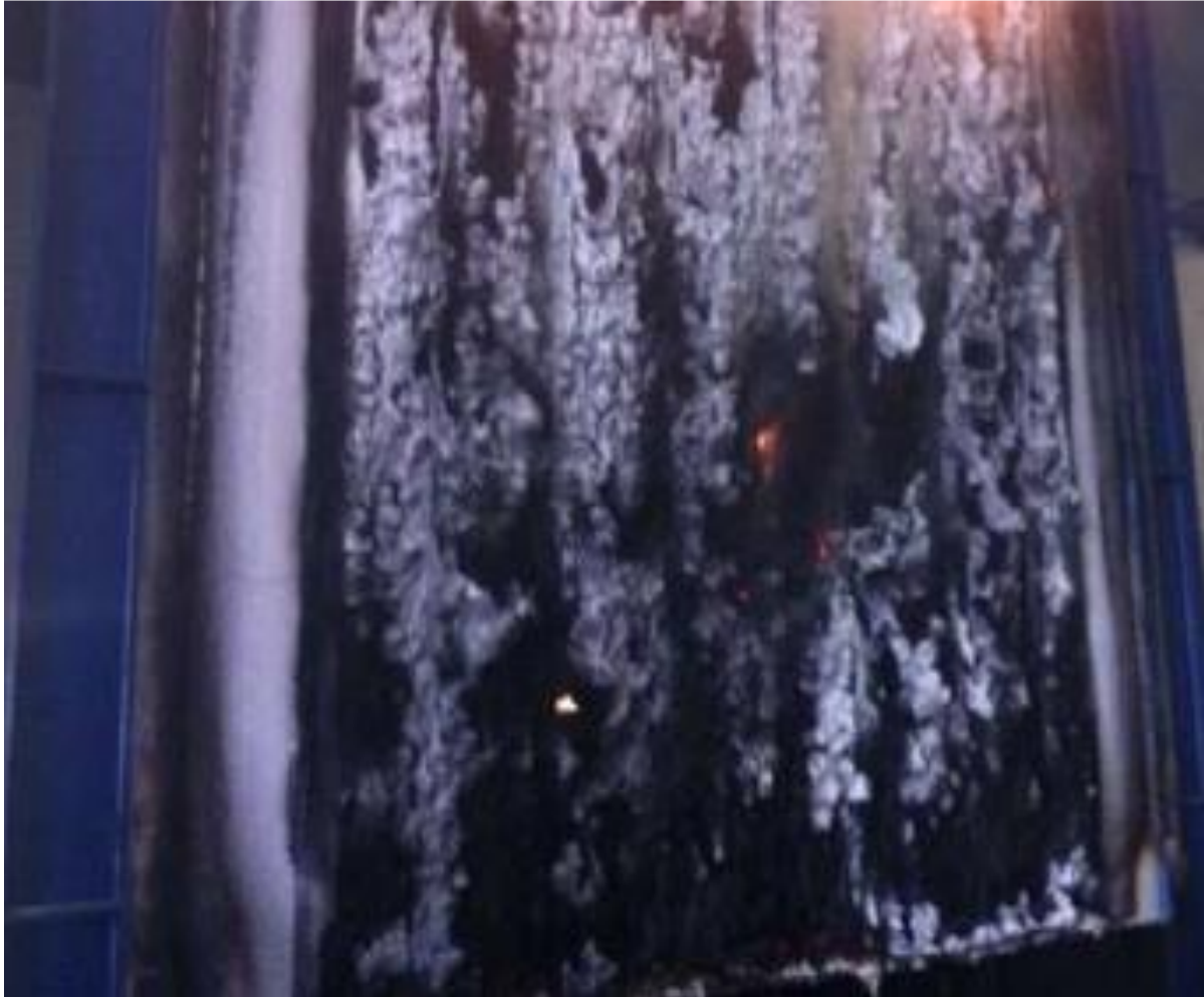
Exposed Face After the Fire Test
