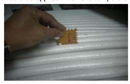
4. Recommended coating thickness on cables: Wet approx. 2.5mm resulted in 1.6mm dry coating to meet Factory Mutual (FM) approval requirements for the protection of cables. Measuring the DFT by using caliper after fully curing.
